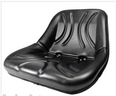
Pan Type Seat Water Drainage System
